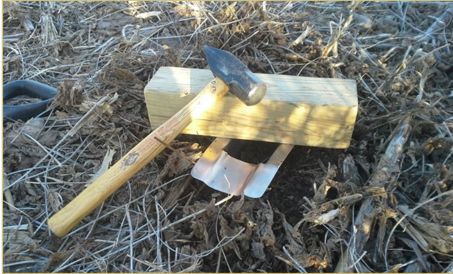
Wood block and small sledge for driving the cutter into harder soils
