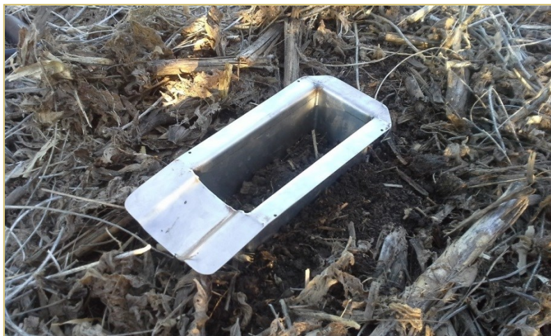
Soil cutter placed on soil surface after residue removal
